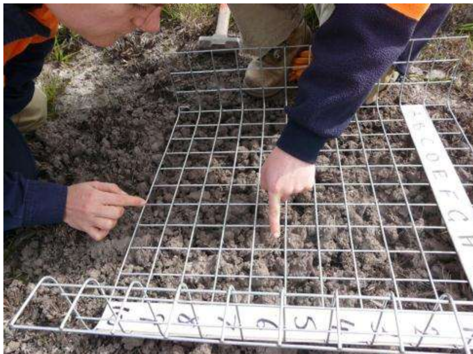
Figure 11 Monitoring grid in use. Grid is constructed from a folded fencing panel with heavy-duty tape. The grid is also marked on the reverse, allowing it to form a raised grid approximately 15cm above the ground to allow it to be used on larger plants.
